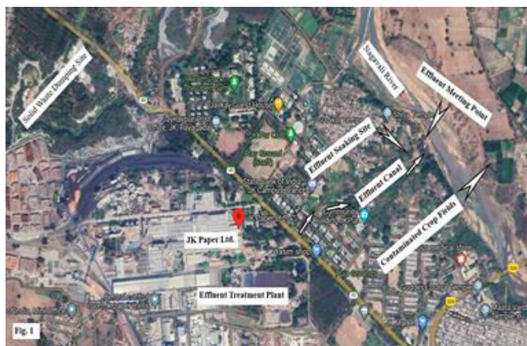
Fig. 1: Google photomaps showing JK Papers Ltd., Effluent canal (Site-SS), effluent soaking open site, effluent joining Nagavalli River and nearby crop fields contaminated by effluent and effluent mixed river water.
